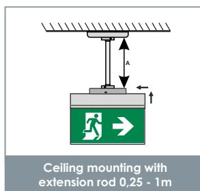
Ceiling mounting with extension rod 0,25 - 1m
