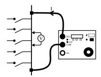
Measuring resistance at busbar joints
