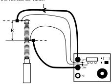
Measuring the resistance of a breaker
